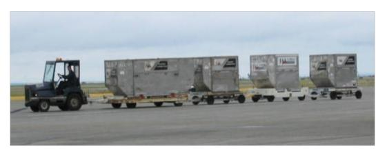
It is strongly recommended that operators tow a maximum of 3 unit loading devices whenever possible.
