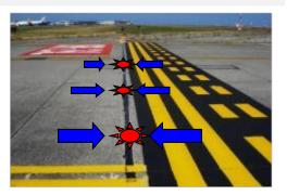
AIRSIDE SAFETY: It is prohibited for a pedestrian, aircraft, or vehicle to cross an illuminated stop bar.
