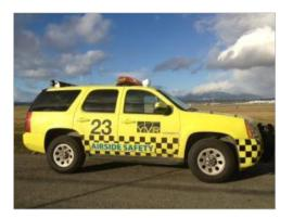
In addition to the vehicle beacon and marking requirements, vehicles operating in the controlled area must display approved identification numbers on each side.
