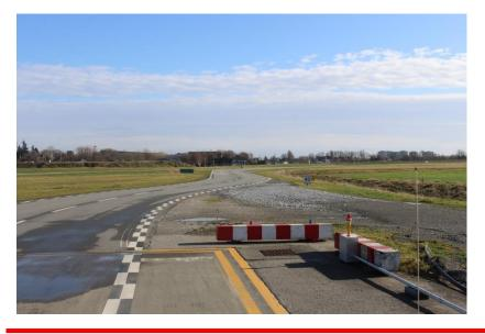
AIRSIDE SAFETY: Aircraft taxi lights will be operational prior to entering the intersection of the Helijet Apron with Taxiway Foxtrot (F). Illuminated lights indicate that the aircraft is ready to start taxiing to Helipad C or down Taxiway F, either by own power or under tow.
